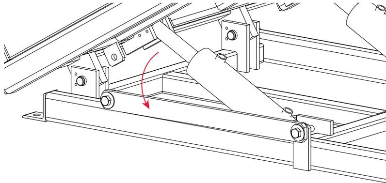
5. Press and hold the **DOWN** button to lower the tilt table to ground or lowest height position then release the button.
