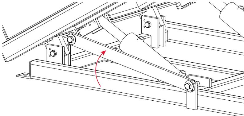
6. Press and hold the **DOWN** button to lower the tilt table until the Maintenance Struts are fully braced against the lower frame of the tilt table.
