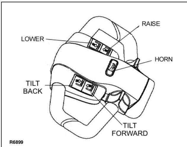
**Figure 2-4. Pushbutton Switches**
