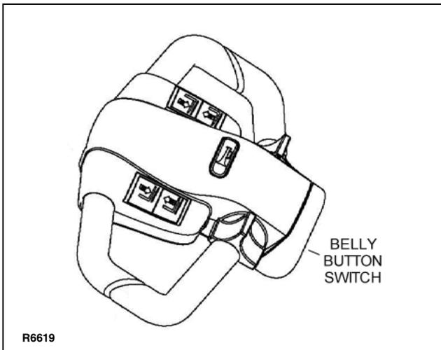
**Figure 2-6. Belly-Button Switch**
