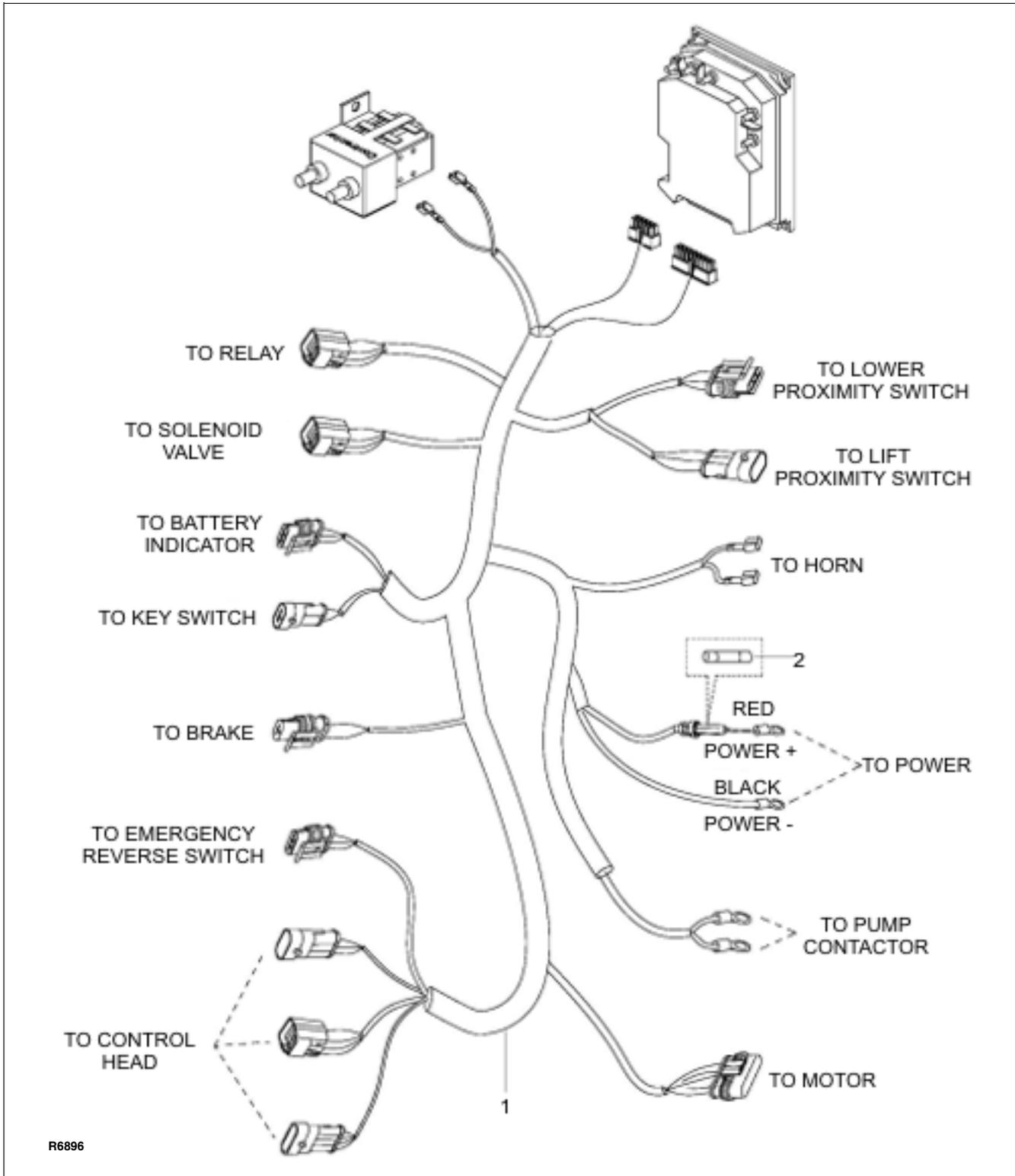
Figure 12-25 Wiring Harness
